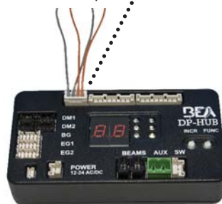
Door Mounted Sensor needs inhibited automatically by DP-Hub or manually
