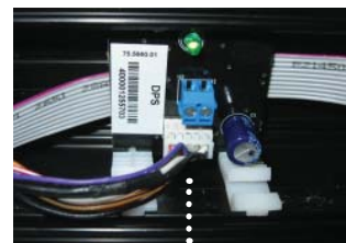
10 pin plug from Door Mounted Sensor Cable
